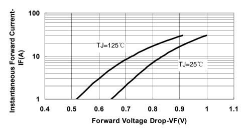
Fig.3-Typical Instantaneous Forward Voltage Characteristics
